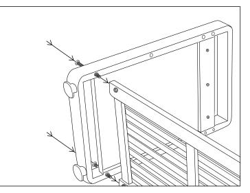
2.Bolt go through frame to get the barrel nut thread.
