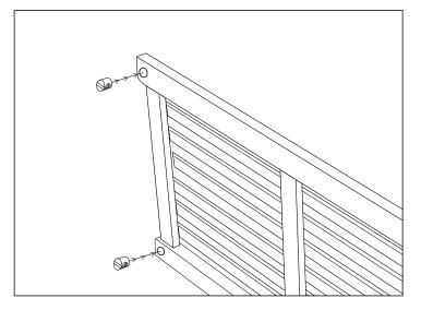
1.Insert barrel nut with threads facing where bolt will enter from the other side
