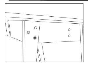
**IF NOT**, it may happen the situation that seems like screw holes are not aligned and the 3rd screw is unable to screw in.
